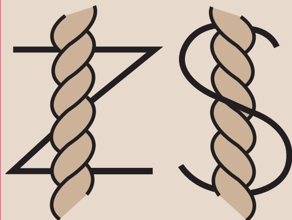
Figure 5 – Left or Z-twist and Right or S-twist.
