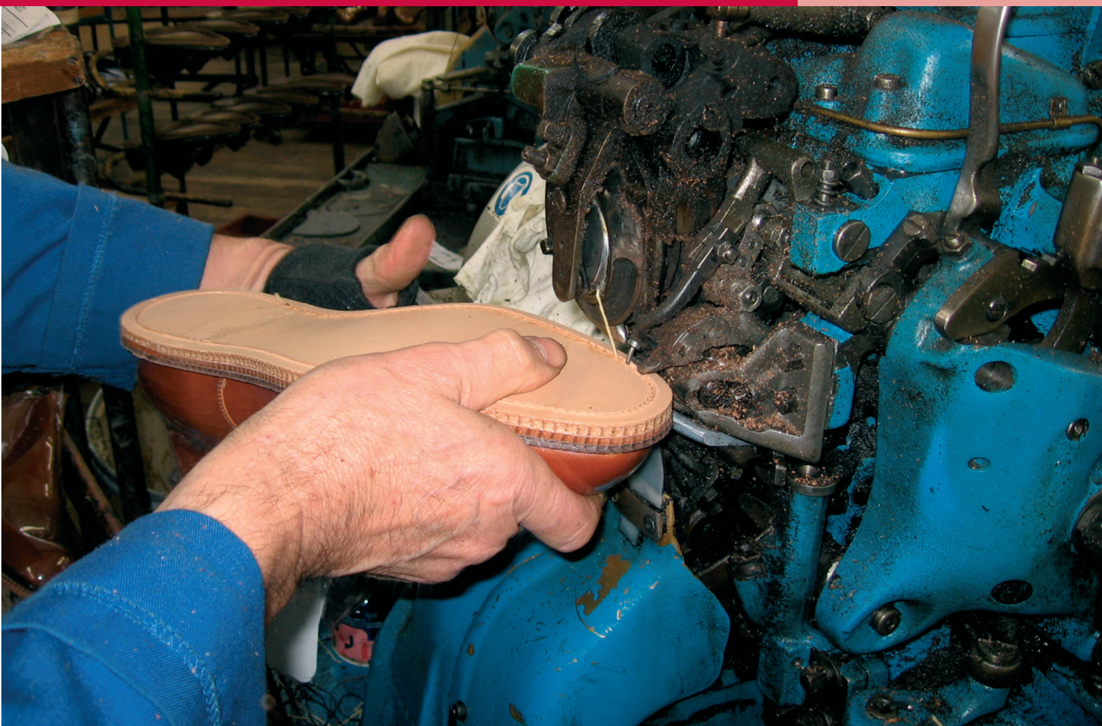
Sole stitching in a groove.
