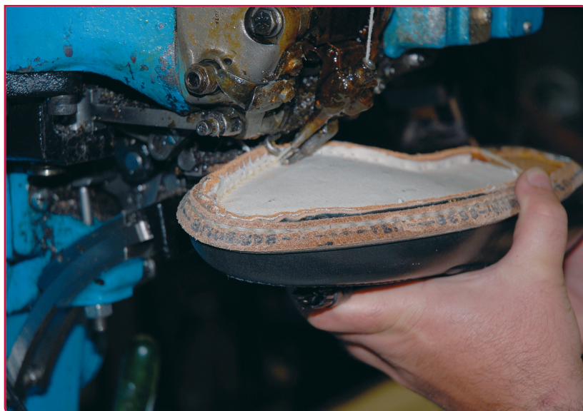
Sewing in a welt. CREDIT: CHURCH &amp; CO (FOOTWEAR) LTD
