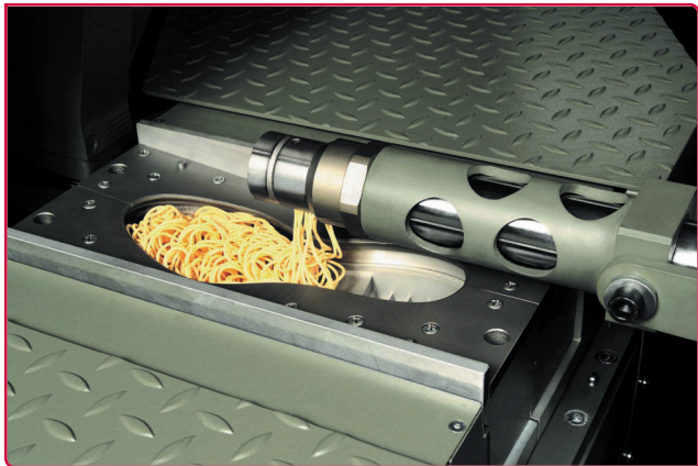
Injecting a ribbon of VR into the mould. CREDIT: DESMA
