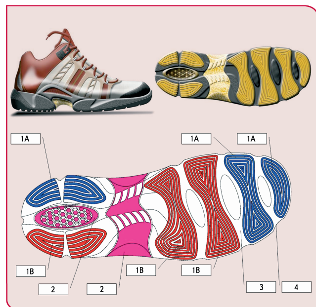
Typical multi-colour TPU sole design that can be produced by multi-injection and casting on a direct moulding machine.
