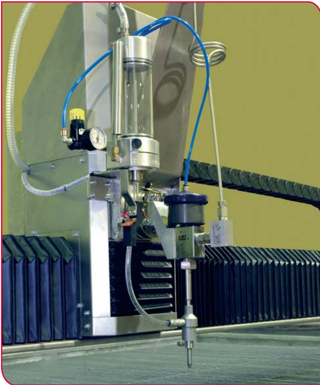
The operating head on a water jet cutter has no direct contact with the material CREDIT: ZIPOR S.A.
