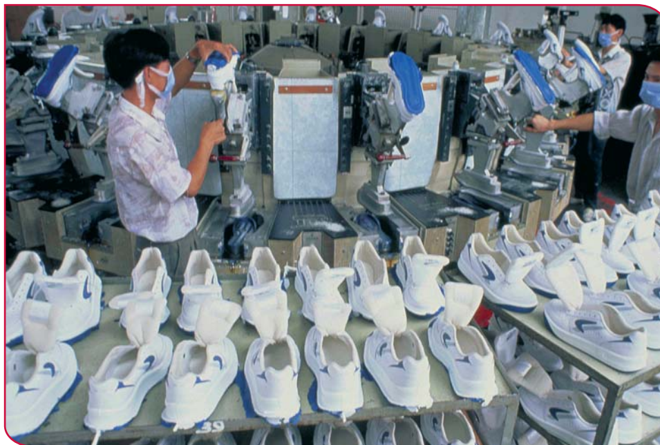
PU/PU direct moulding on sports shoes. CREDIT: STEVE LEE
