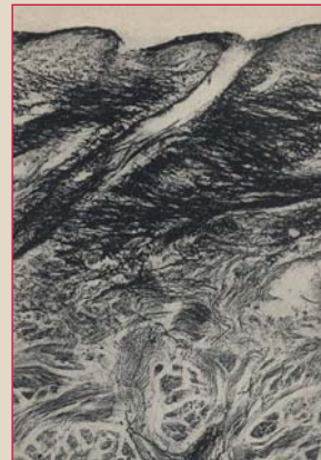
Cross-section of grain layer of calf hide after hair removal. (Section sampled from the butt area, 20 microns magnification 140 diametres.)
