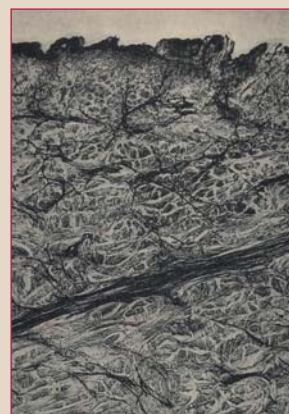
Cross-section of grain layer of pig skin after hair removal. (Section sampled from the butt area, 20 microns magnification 140 diametres.)
