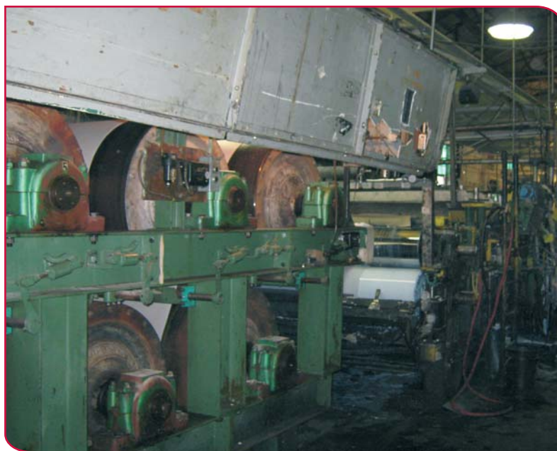
After wet web saturation created the foundation of the board, it is partially dried, the all-important latex binder added, followed by further drying and curing to produce the final board. CREDIT: BONTEx
