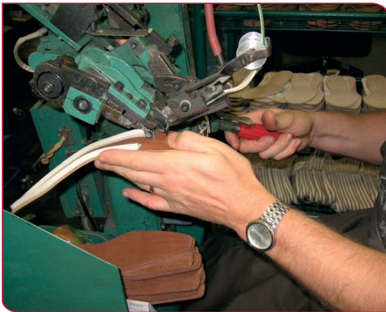
Applying a rib (the importance of this operation is not always appreciated by manufacturers new to the Goodyear welted construction)
