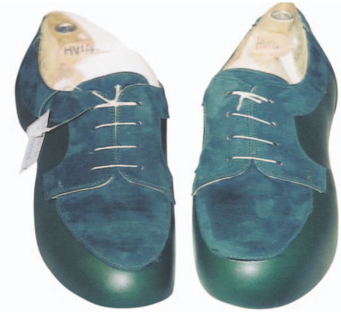
Figure 3: Pair of lasted orthopaedic shoes being made for a customer with badly twisted feet.
