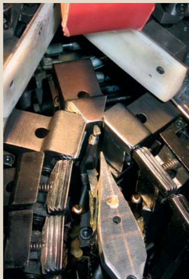
Figure 6: Cerim forepart laster with extra toe post for elongated toes
