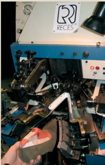
Figure 3: Typical 9 pincer forepart laster from Reces
