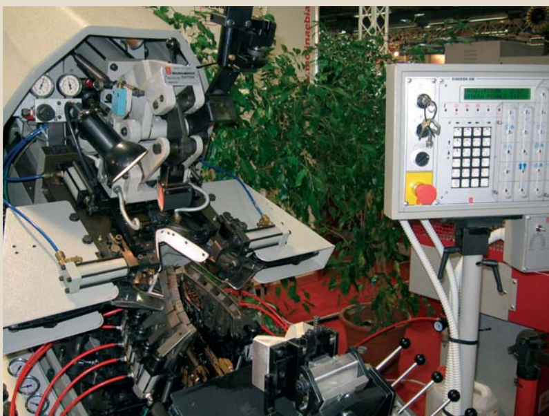
Figure 1: Molina Bianchi Sincron 11 pincer forepart laster
