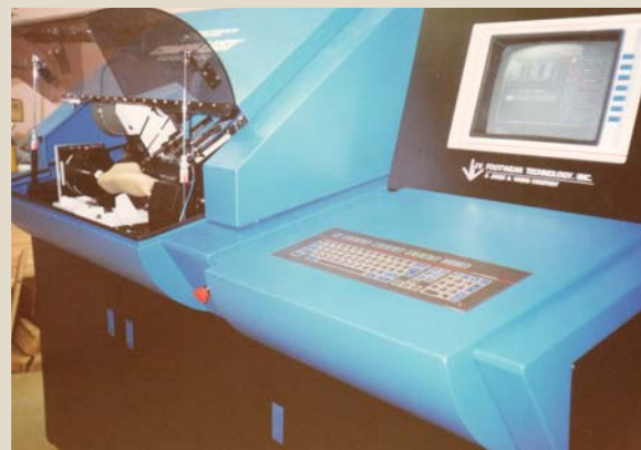
Compu-Last CL-300, the first combined last digitiser/lathe for prototypes (1991)
