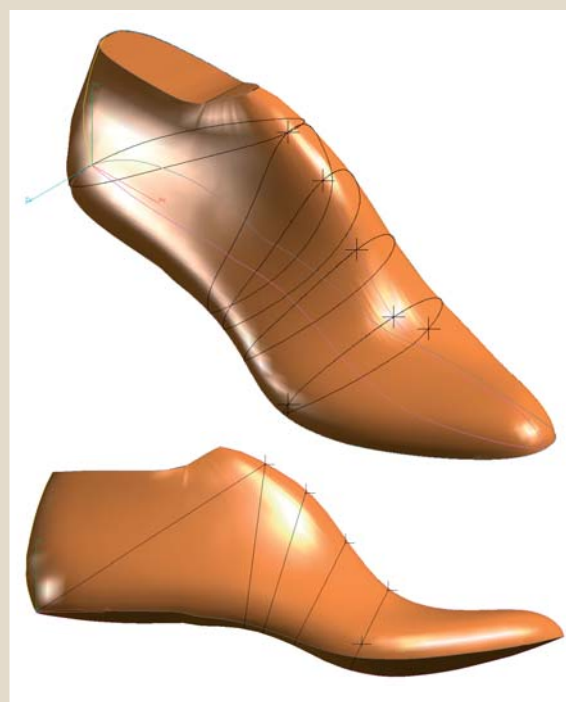
Girth sections from Lectra's Romans CAD software showing the different shapes of the measurements showing why they should not all have the same girth grade
