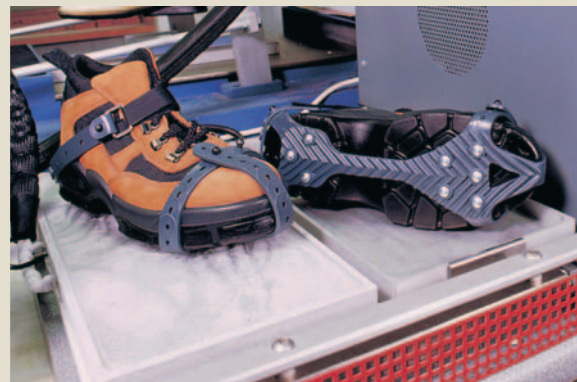
Slip test using an ice tray
