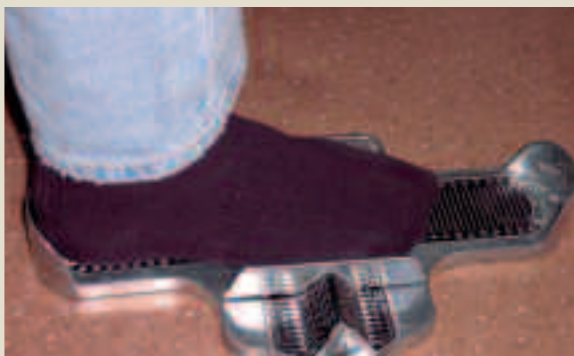
Brannock foot measuring device
