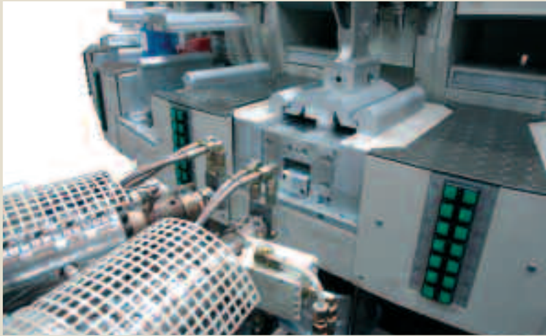
Mould and two Desma injection heads
