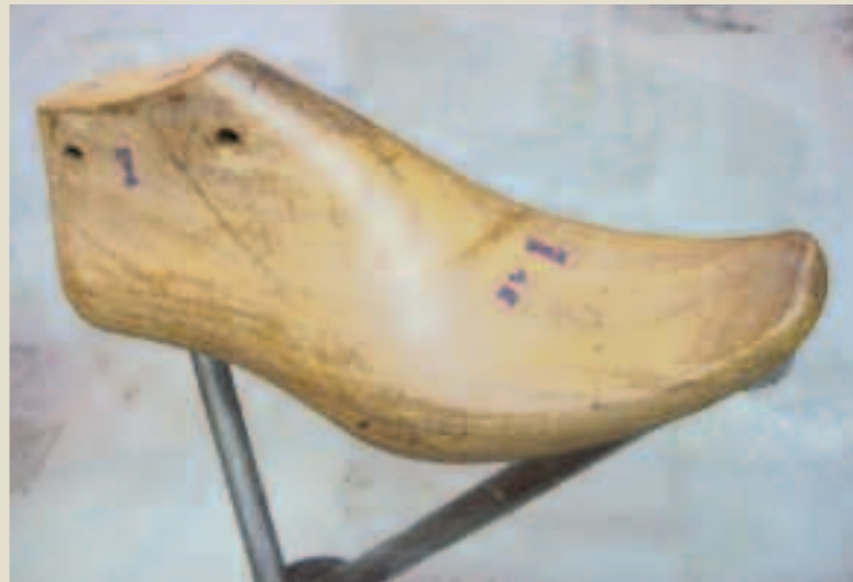
The scoop block system used by Ashoke Kumar and other Agra last makers provides easy last slipping
