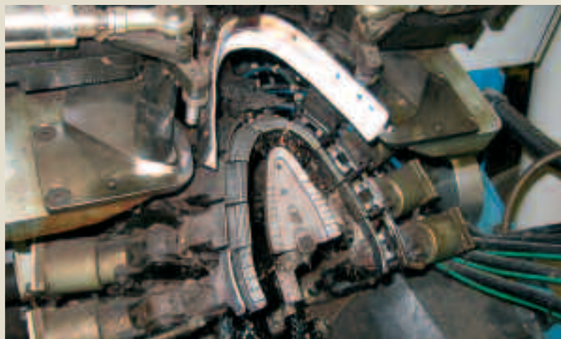
Figure 3: Vertical rib centre block on a USM machine
