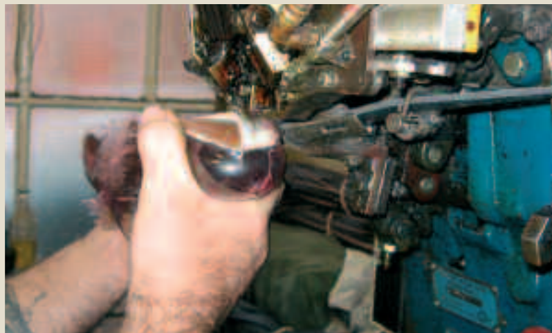
Figure 4: Approaching the toe in welt-sewing
