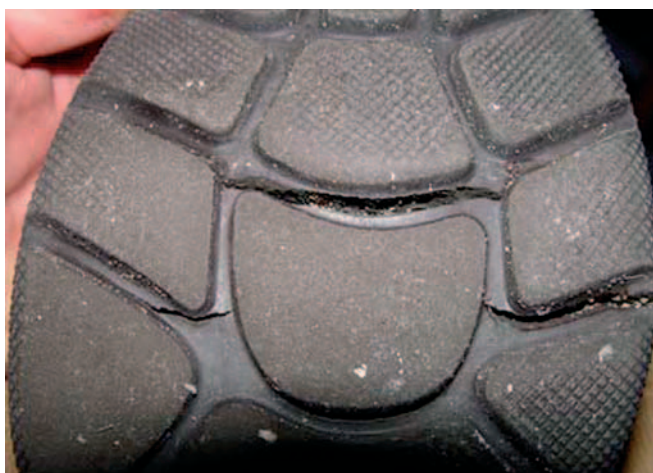
Figure 1: Typical example of sole cracking
