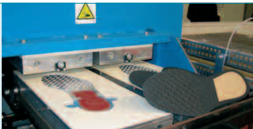
Euromeccanica's sole embossing equipment showing embossed sole
