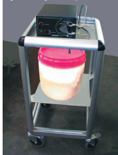
Figure 2: Dosing unit for liquid colours
